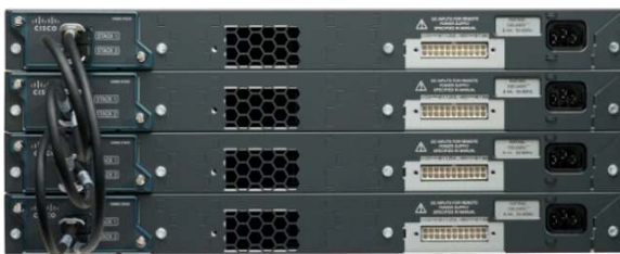
Figure 3. Cisco FlexStack Module and Switches
